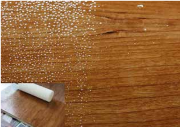
Fig 2. Defoaming properties of BYK-1799 (right), used at 0.05% based on the total formulation compared with the system without defoamer (left) for a 100% UV-curing clear coat system applied using a moltopren roller
