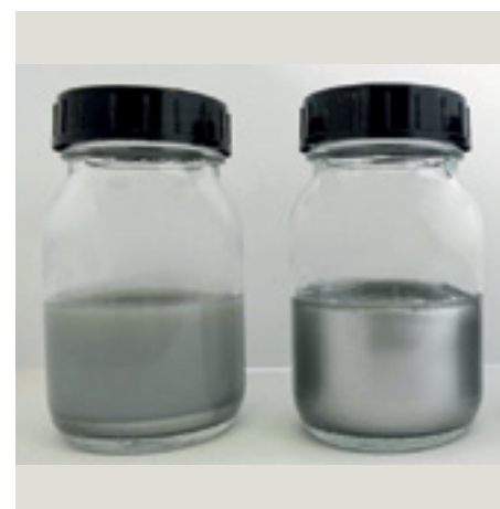
Figure 5: Anti-settling behaviour of a water-borne 2-pack polyurethane aluminium basecoat, without (left) and with (right) a polyamide additive (aluminium pigment: "Eckart Hydrolan IL 2154").
